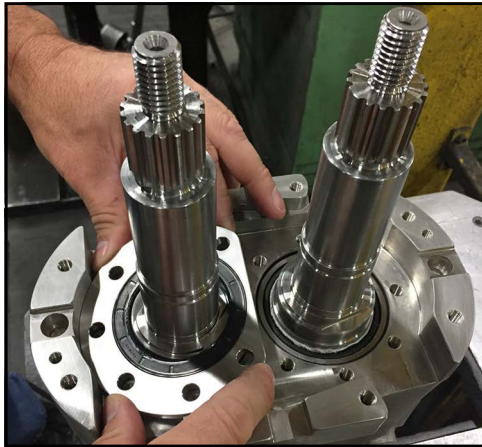
Figure 157 - Remove bearing retainer
