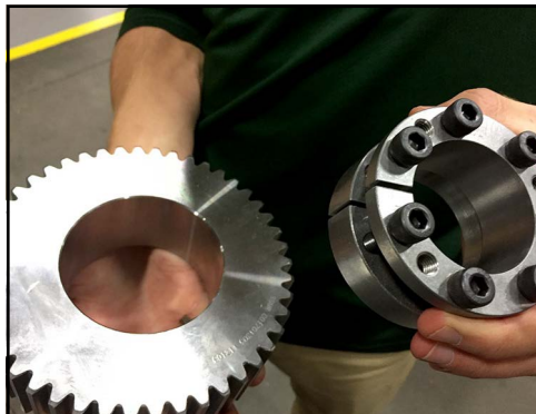
Figure 222 - Assemble locking assembly into gear
