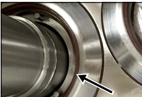
Figure 49 - Remove carrier-to-seal O-ring
