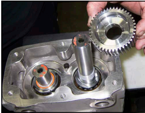
Figure 213 - Install drive gear
