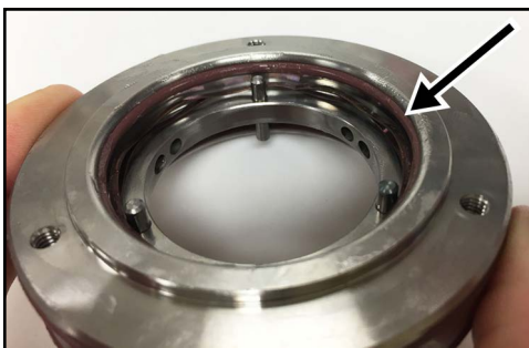
Figure 75 - Carrier-to-seal O-ring installed
