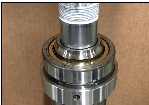
Figure 180 - Press race into bearing
