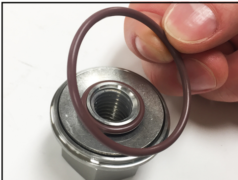
Figure 119 - Install screw nut O-ring
