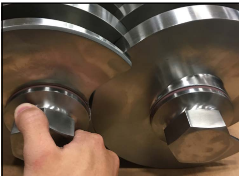
Figure 127 - Install screw nuts
