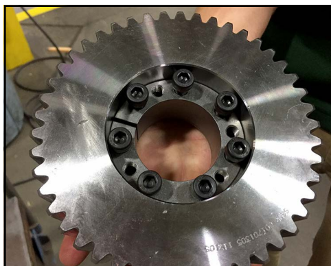
Figure 223 - Place locking assembly into gear
