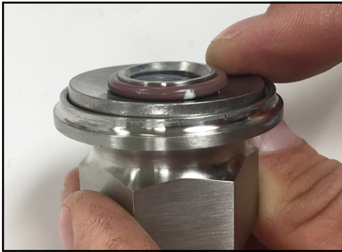
Figure 118 - Belleville washer installed
