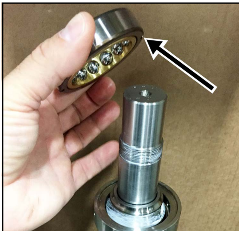
Figure 176 - Place bearing onto race
