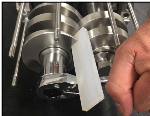
Figure 230 - Tighten screw nut
