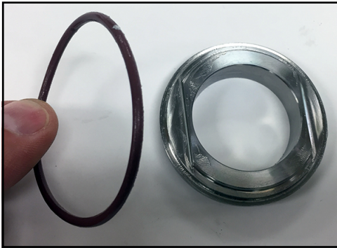
Figure 46 - Remove cap-to-seat O-ring
