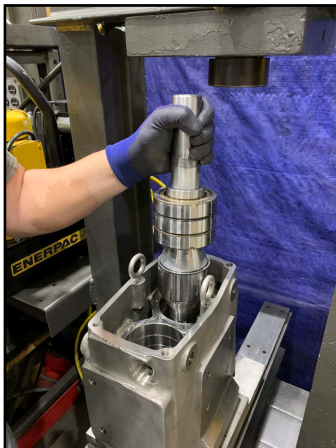
Figure 305 -Place drive shaft in bore
