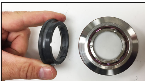
Figure 76 - Lubricate and install seal
