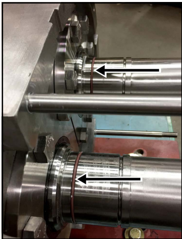
Figure 137 - Install shaft O-rings
