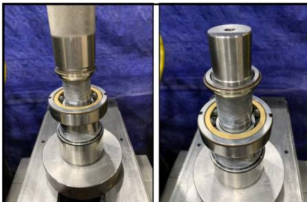
Figure 284 -Place race on shaft
