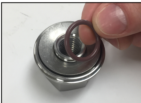
Figure 117 - Install washer retainer O-ring
