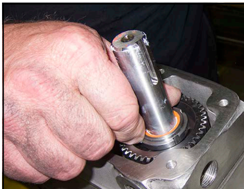
Figure 216 - Install locking nut
