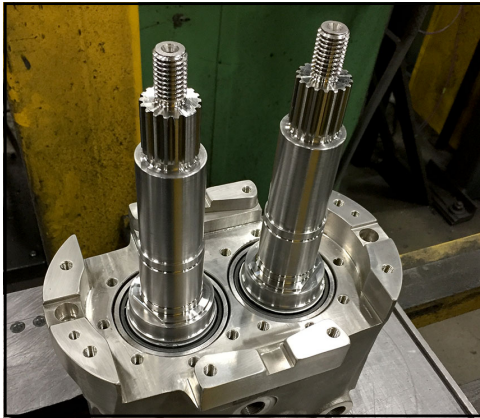
Figure 202 - Shafts seated in gearcase
