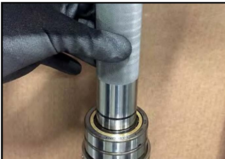
Figure 287 -Press race onto shaft
