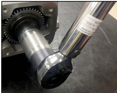
Figure 154 - Loosen locking nut
