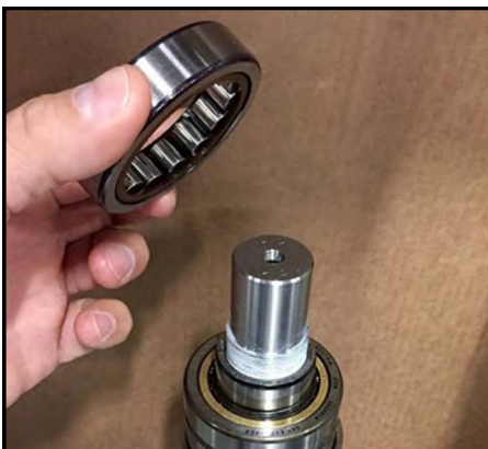
Figure 288 -Place bearing onto race
