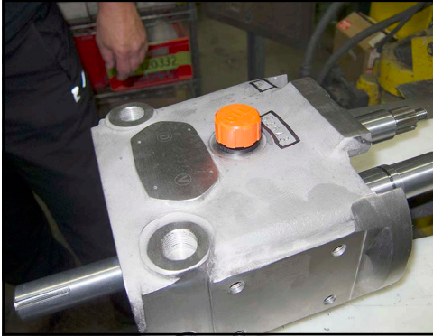
Figure 219 - Install oil breather plug
