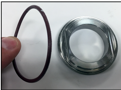
Figure 100 - Install cap-to-seat O-ring
