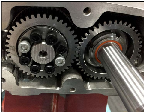
Figure 225 - Align loose gear with drive gear
