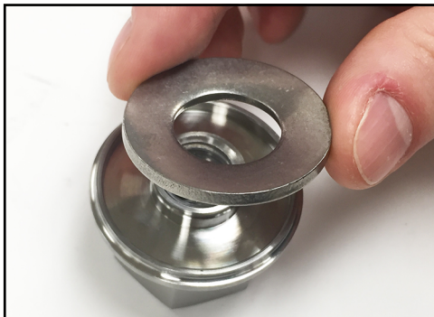
Figure 116 - Install belleville washer
