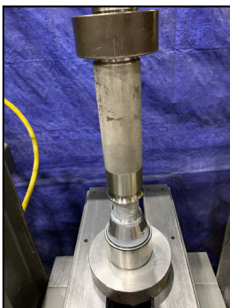
Figure 281 -Press race onto shaft
