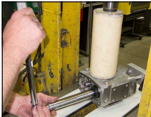
Figure 218 - Torque locking nut
