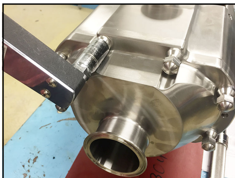
Figure 135 - Torque cover nuts
