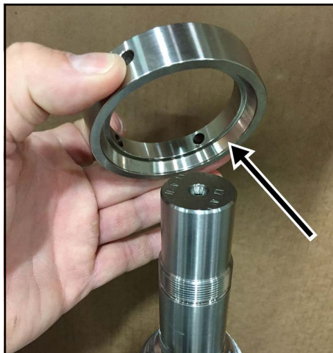
Figure 168 - Place bearing spacer on shaft
