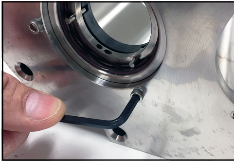
Figure 56 - Remove cap screws
