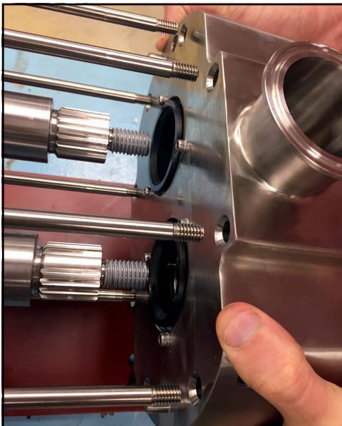
Figure 90 - Install pump body onto shafts
