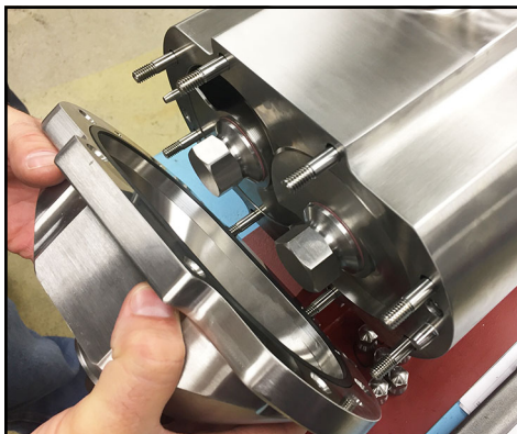
Figure 131 - Install pump cover
