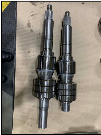
Figure 302 -Shaft ready to be installed
