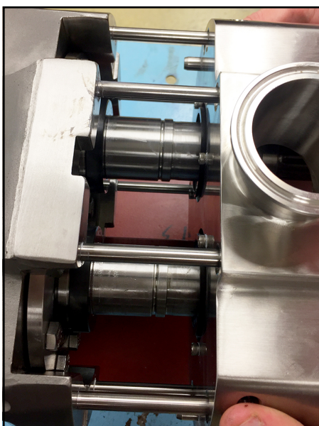
Figure 65 - Remove pump body-ported
