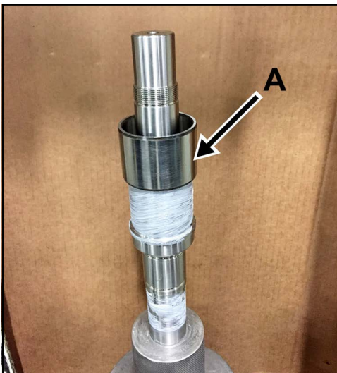
Figure 165 - Place inner race on shaft
