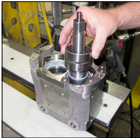
Figure 198 - Place outer race on shaft
