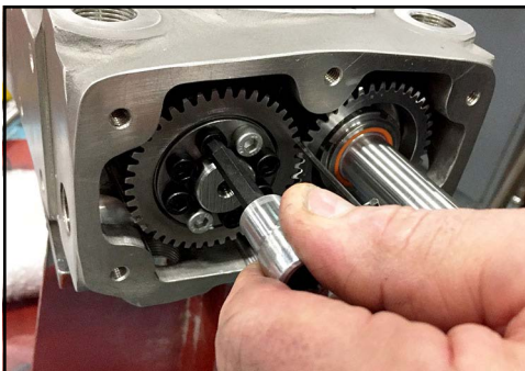
Figure 256 - Loosen bolts in locking assembly
