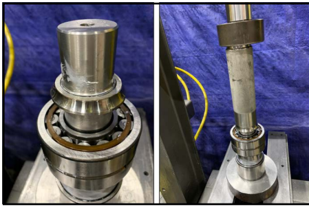
Figure 289 -Place race on shaft
