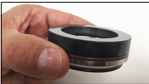
Figure 105 - Seal seat installed on seal cap
