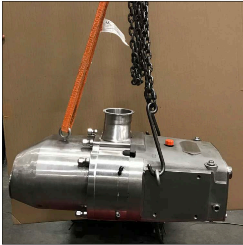
Figure 3 - Lifting location - 130, 220-UTS
