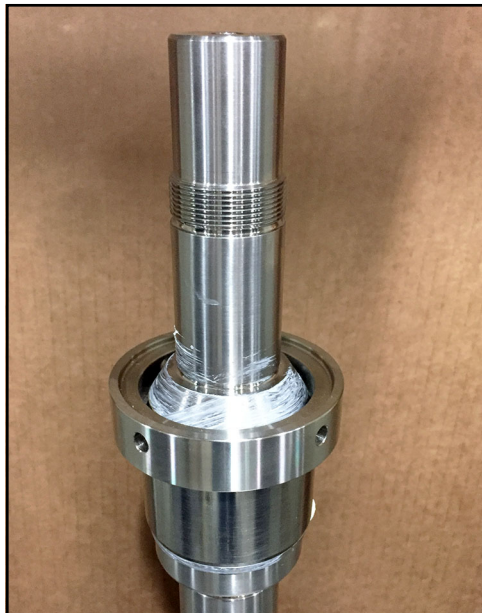
Figure 169 - Bearing spacer installed
