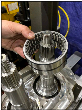
Figure 313 -Place outer race on the shafts
