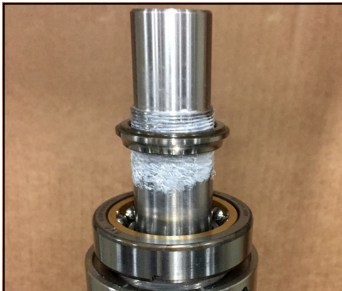
Figure 182 - Place race on shaft
