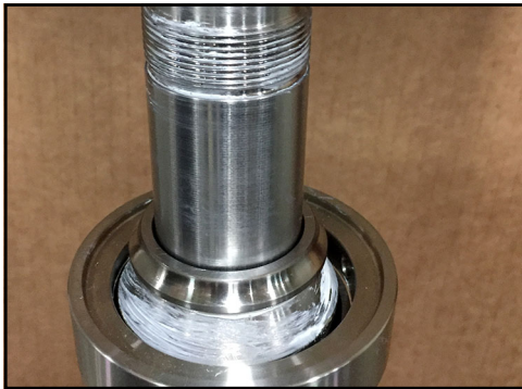
Figure 175 - Race pressed on shaft
