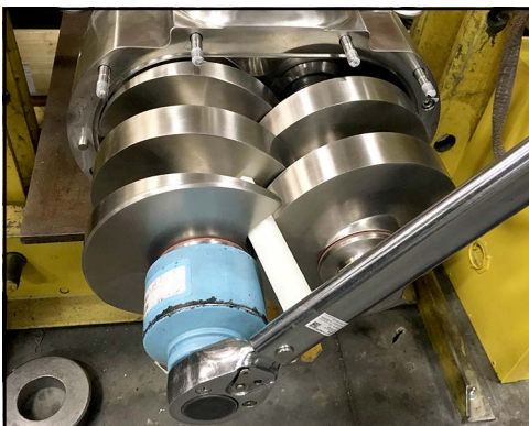
Figure 128 - Torque left screw nut
