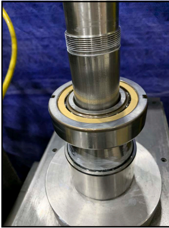
Figure 285 -Race installed on shaft
