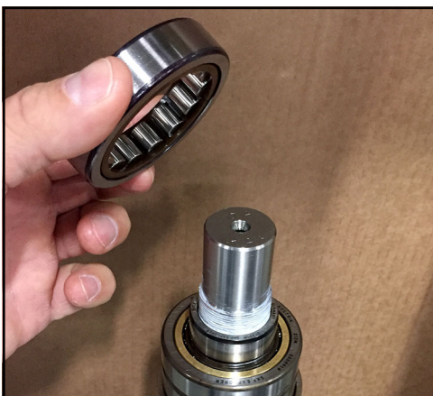
Figure 188 - Place bearing onto race
