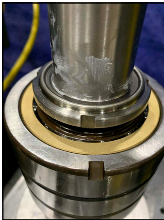
Figure 297 -Place locking nut on to shaft
