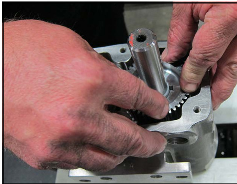
Figure 214 - Install drive gear
