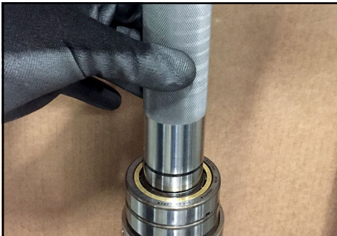
Figure 187 - Press race onto shaft
