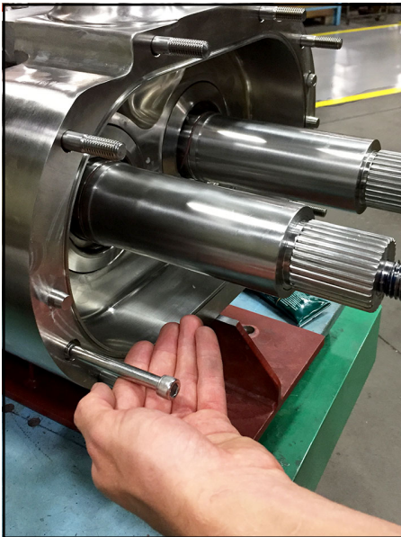
Figure 143 - Install body retaining screws
