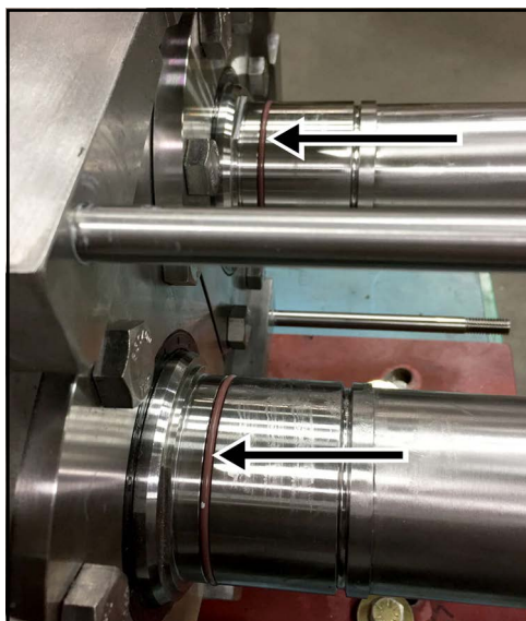
Figure 87 - Install shaft O-rings
