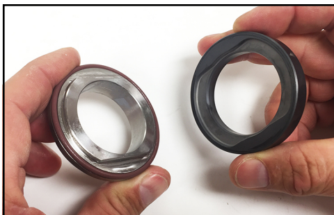
Figure 44 - Remove seal seat from seal cap
