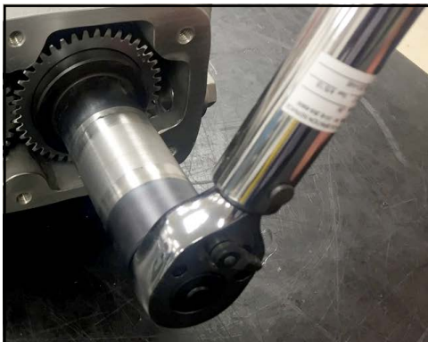
Figure 260 - Loosen locking nut
