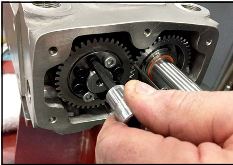
Figure 150 - Loosen bolts in locking assembly
