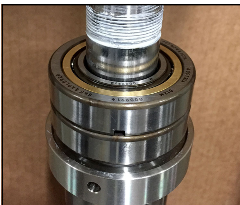
Figure 184 - Second bearing installed
