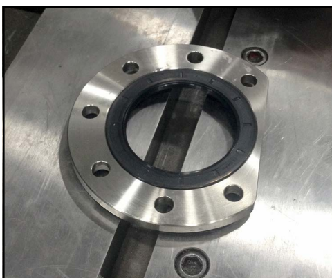
Figure 205 - Bearing retainer seal installed
