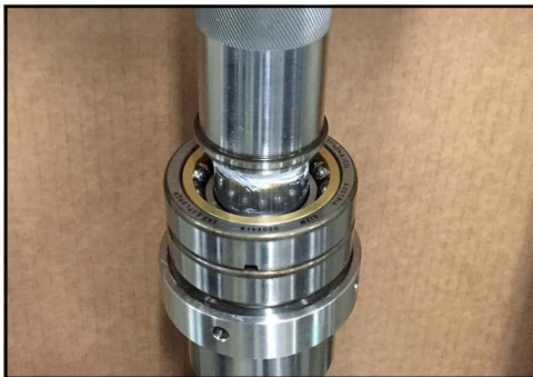
Figure 183 - Press race into bearing
