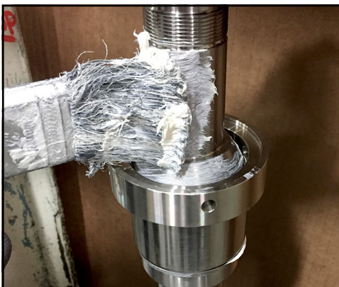
Figure 172 - Apply anti-seize to shaft
