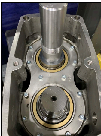
Figure 312 -The rear bearing retainer bolts
