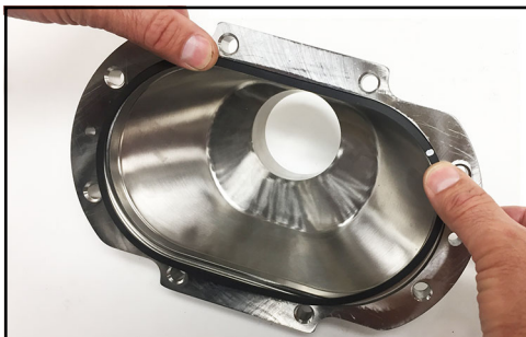
Figure 29 - Remove cover gasket
