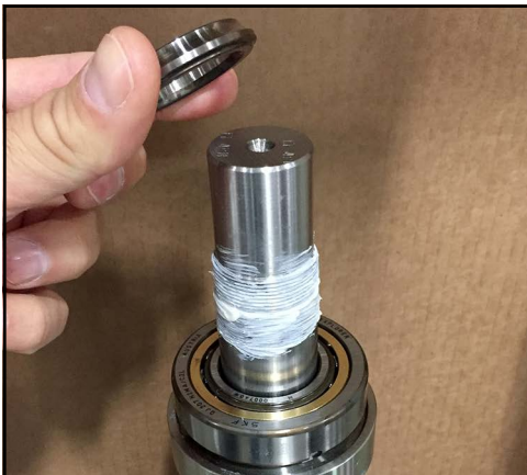
Figure 179 - Place race on shaft
