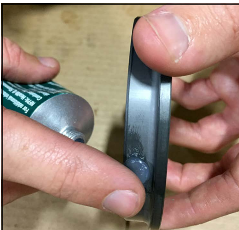
Figure 84 - Lubricate the outer diameter of the seal
