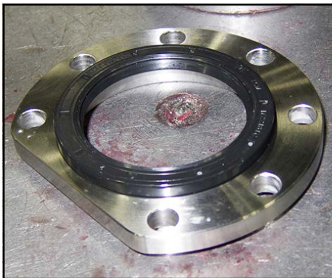
Figure 203 - Center bearing retainer seal
