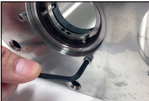
Figure 83 - Install with cap screws
