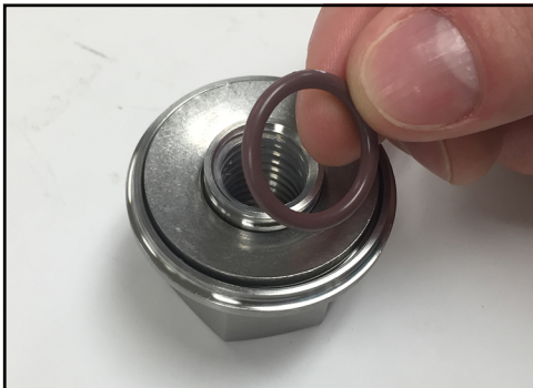
Figure 39 - Remove washer retainer O-ring
