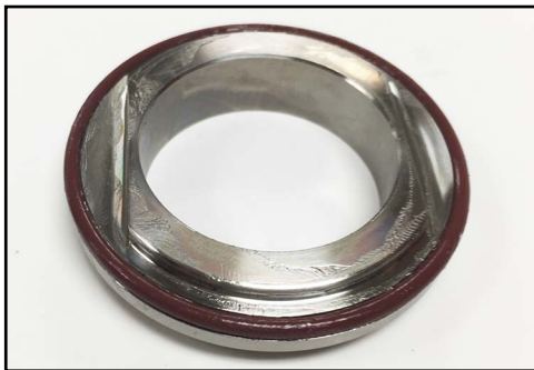
Figure 101 - Cap-to-seat O-ring installed
