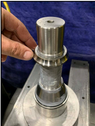
Figure 280 -Place race onto shaft
