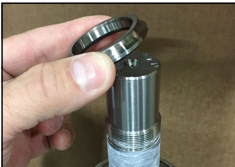
Figure 173 - Place race onto shaft
