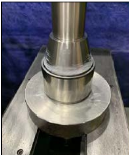
Figure 276 -Inner race installed on shaft
