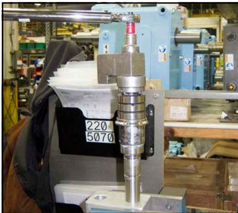
Figure 190 - Torque down locking nut
