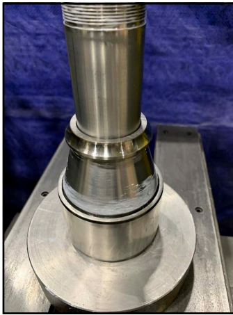
Figure 282 -Race pressed on shaft
