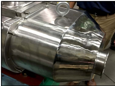
Figure 133 - Seat pump cover against pump body
