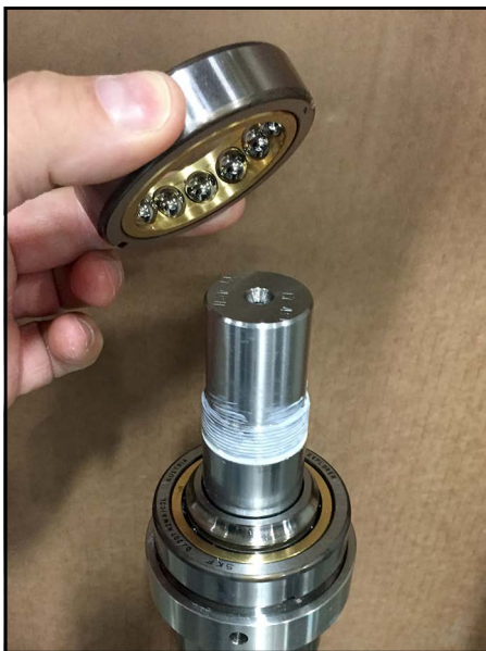
Figure 291 -Place bearing onto race
