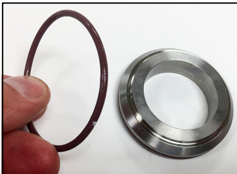
Figure 45 - Remove cap-to-screw O-ring
