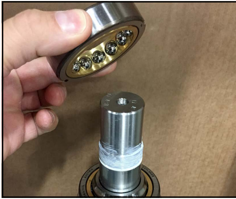
Figure 181 - Place bearing onto race
