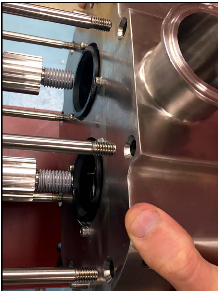
Figure 140 - -Install pump body onto shafts
