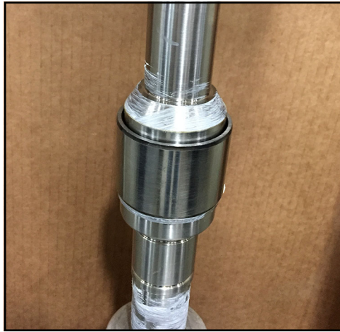
Figure 167 - Inner race installed on shaft
