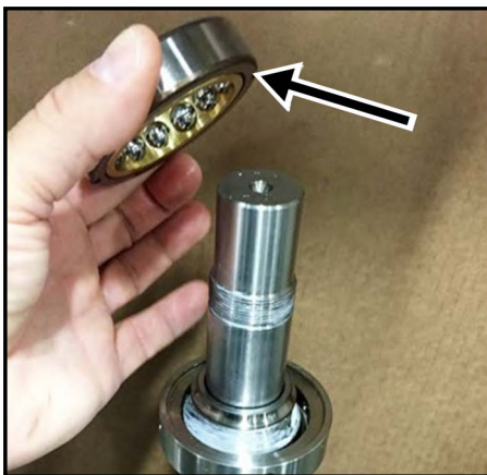
Figure 283 -Place bearing onto race
