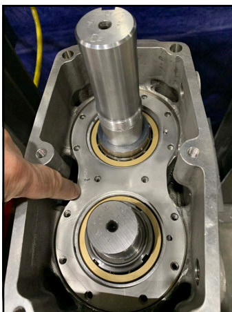
Figure 309 -Rear bearing retainer plate
