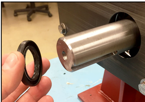
Figure 249 - Install oil seal
