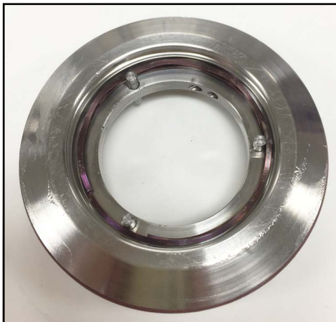
Figure 70 - Seal wave spring installed
