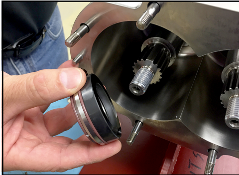
Figure 43 - Remove seal cap assembly
