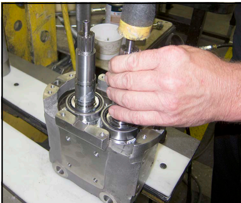
Figure 201 - Tap shafts to center in bores
