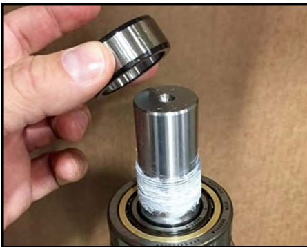
Figure 286 -Place race onto shaft
