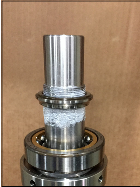
Figure 292 -Place race on shaft
