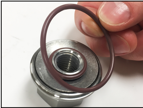
Figure 38 - Remove screw nut O-ring
