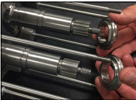
Figure 226 - Install seal caps
