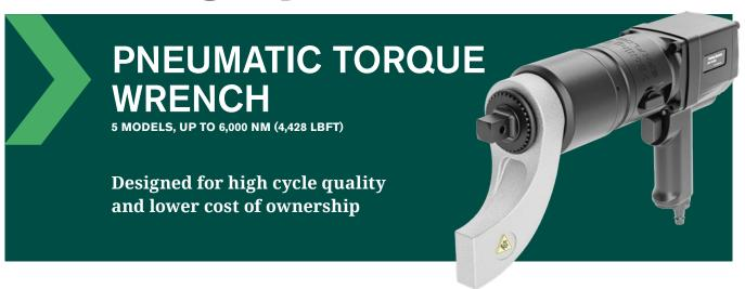
Incorporating a robust planetary gear system driven by a pneumatic motor through a two-speed transmission, our Pneumatic Torque Wrenches offer high speed and accuracy. Each wrench is individually calibrated to establish an accurate relationship between desired torque and corresponding air pressure, resulting in output torque accuracy and repeatability of +/- 3%. Automatic switch-off function at the desired torque aids the user in establishing reliable and repeatable operation.
